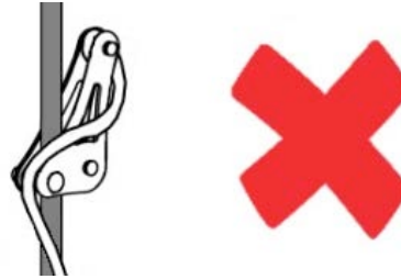
Figure 3: Dangerous result of using a loose or supple tether: Rope Wrench is stuck in neutral position and could release the grip of the friction hitch below it.
